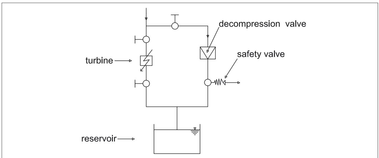
Figure 8. Bypass composed of a decompression valve with a reservoir
