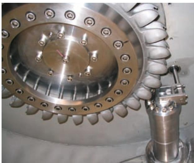
Photo 11. Pelton runner with one nozzle, set on the drinking water of Haut Intyamom (Switzerland) ( $\Delta Z = 502$  m,  $Q_n = 40$  l/s, 163 kW, 2006)
