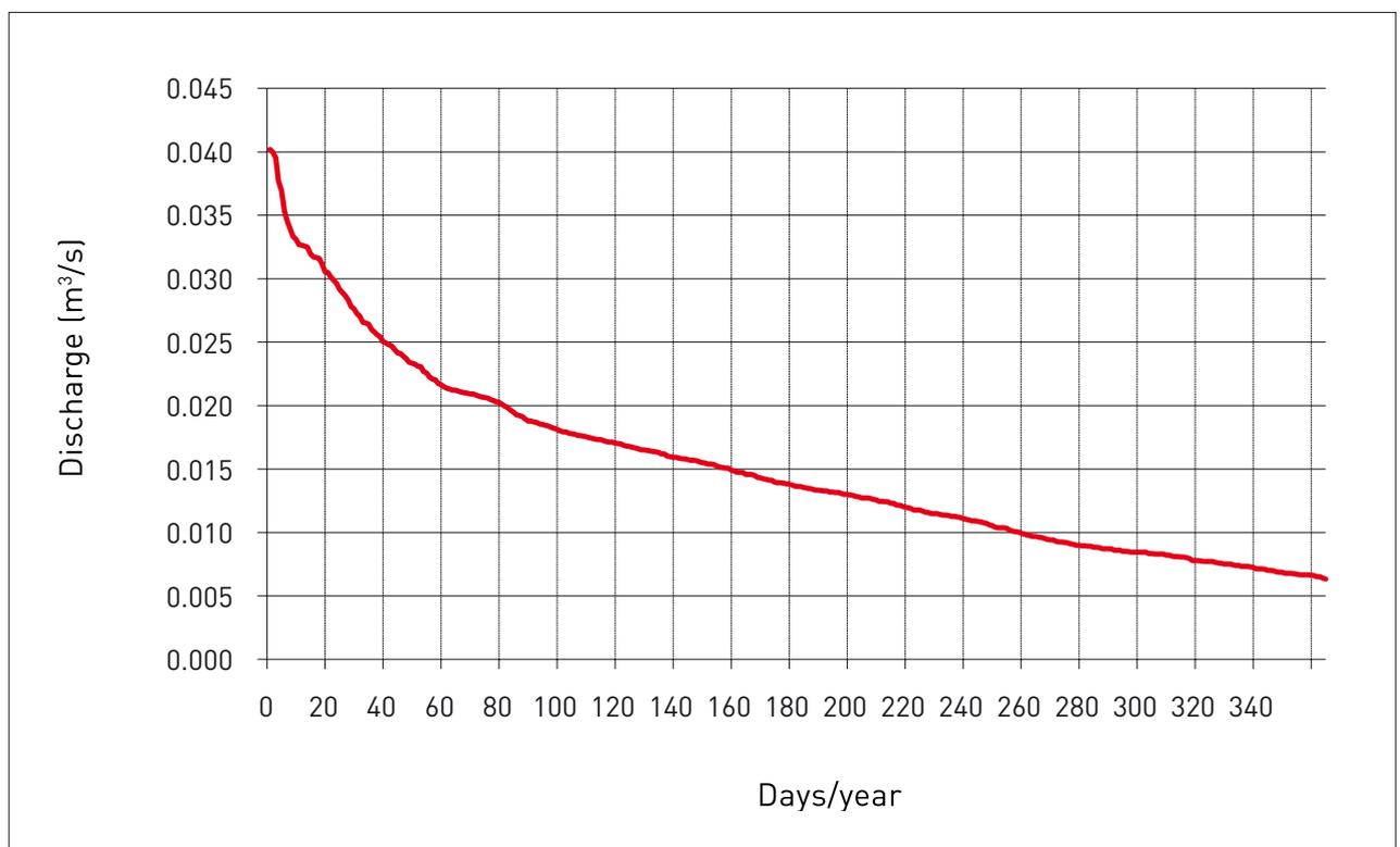
Figure 3. Example of flow duration curve
