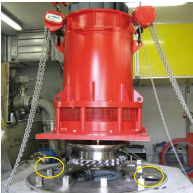
Photo 24. Two open hand holes to reach the deflectors Profray SHP plant (case study n° 11)
