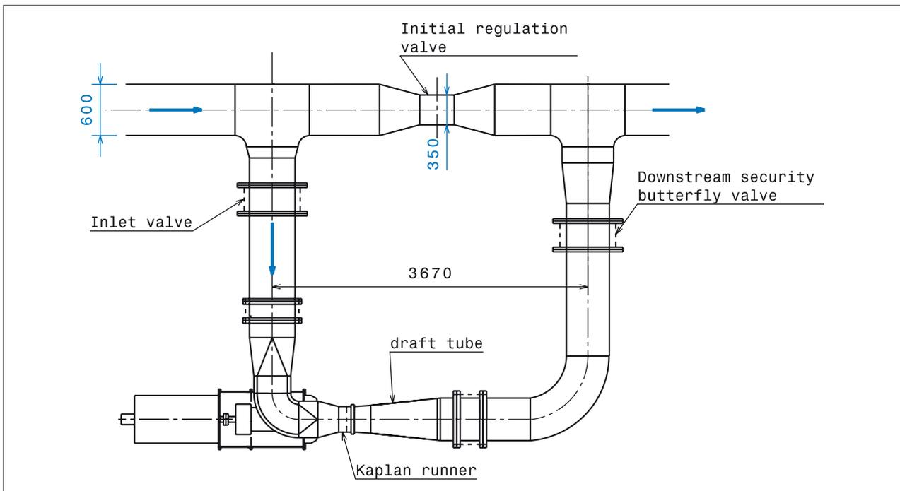
Figure 6. Setting of a Kaplan turbine as a bypass of an existing valve in a drinking water network, Poggio Cuculo SHP plant (case study n°4) (cotations in mm)
