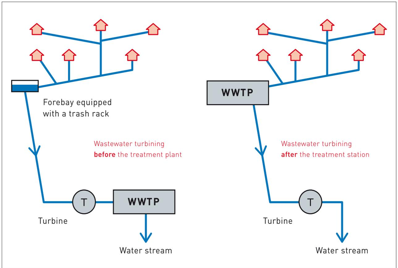
Figure 2. Turbine settings before and after the wastewater treatment plant (WWTP)
