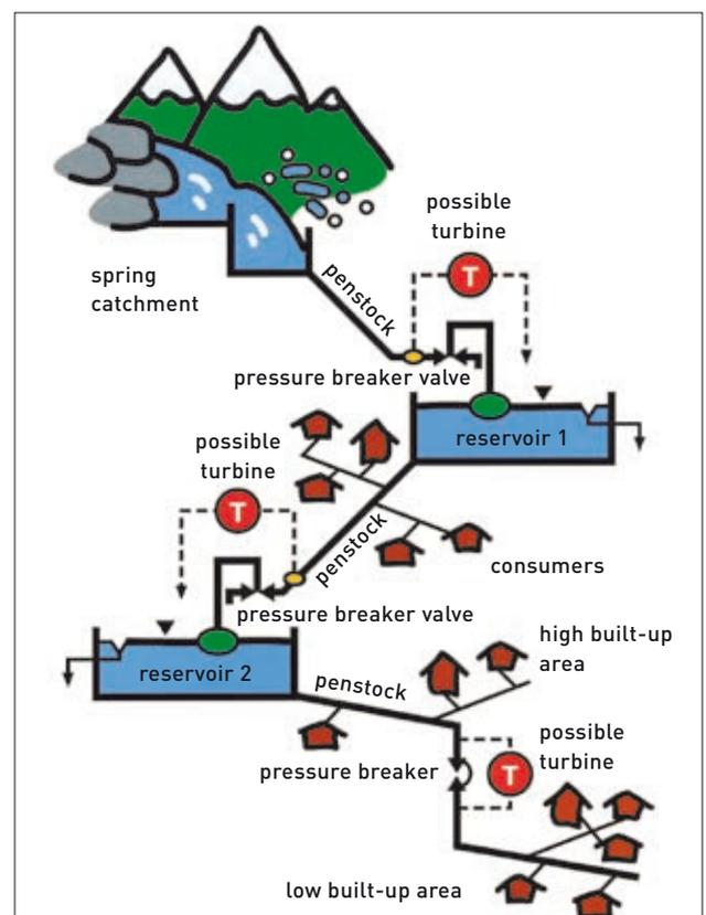
Different energy recovery possibilities can be identified, defined by the turbine positions:
