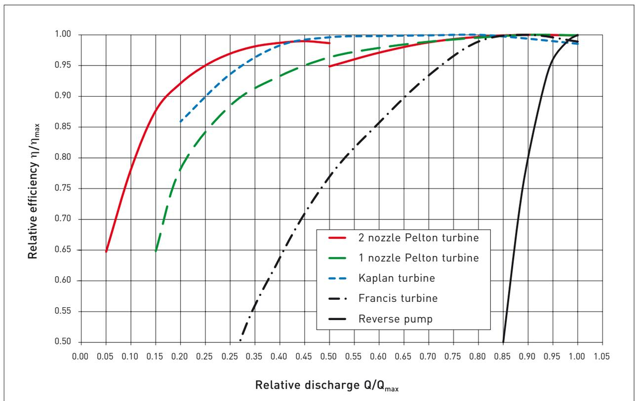
**Figure 4. Evolution of the relative efficiencies regarding the discharges for Pelton, Kaplan and Francis turbines, and reverse pumps**
