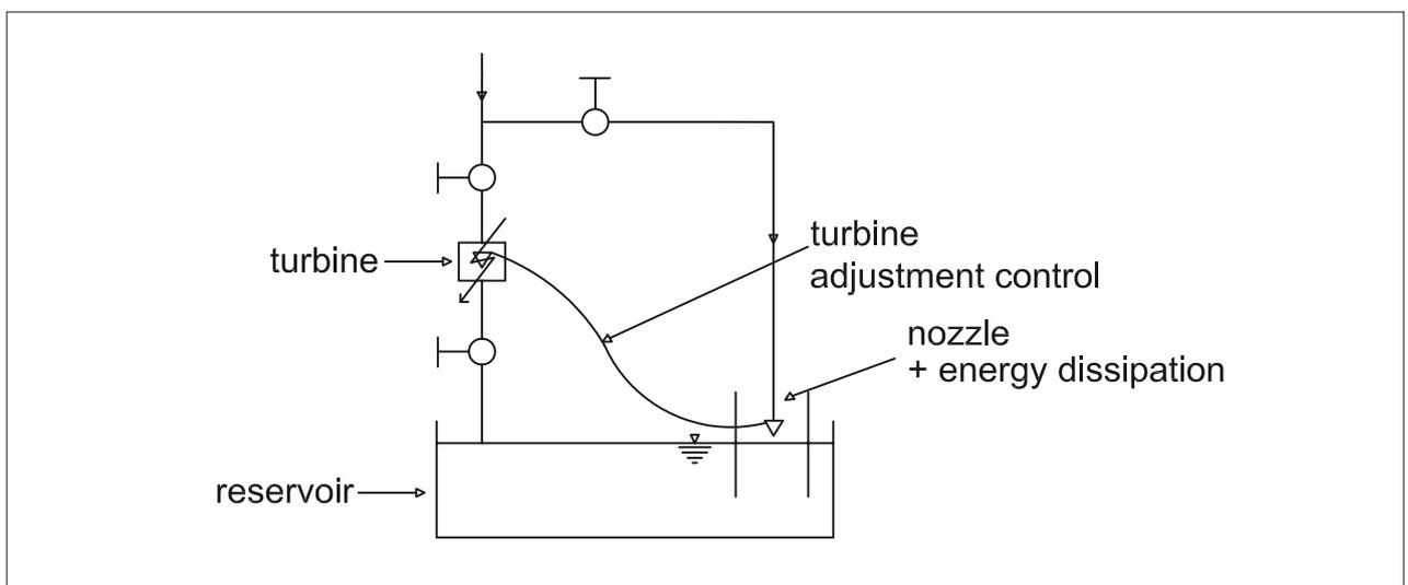
Figure 9. Bypass composed of an adjustable nozzle for high heads
