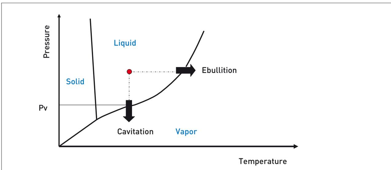
Figure 7. Diagram of the body states and phase change curves <sup>10</sup>
