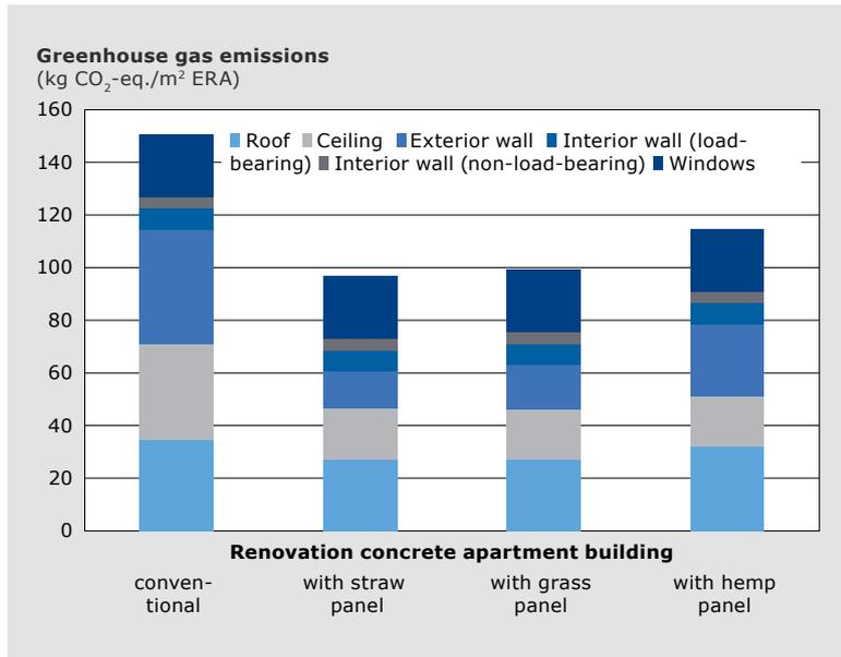
When thermally renovating a concrete building, greenhouse gas emissions are reduced by up to a third by using sustainable insulation materials such as straw, grass or hemp (graphic: ZeroStrat final report, edited).
