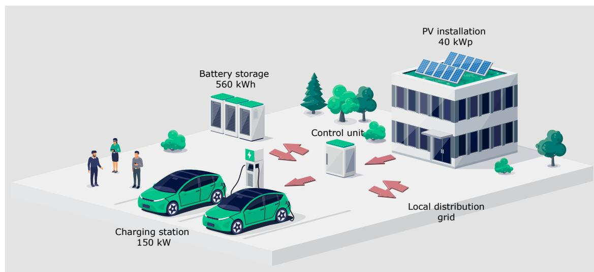
An intelligent control system coordinates the various components of the charging station to minimise the amount of electricity required from the local distribution grid for charging (graphic: B. Vogel / Shutterstock).
