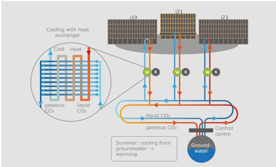
Cooling: When the liquid CO<sub>2</sub> is heated, it vaporises and becomes gaseous. This process releases cold, which can be used to cool buildings (source: HES-SO Valais-Wallis, edited).
