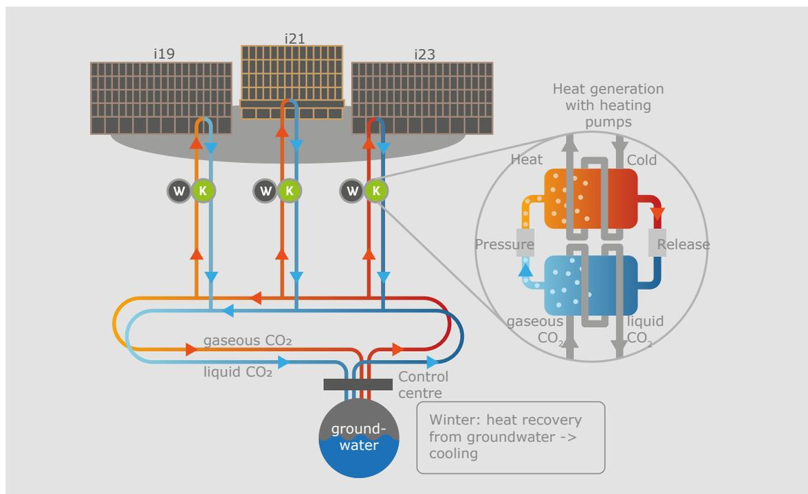
Heating: When gaseous CO<sub>2</sub> cools down, it condenses. This change from gaseous to liquid releases heat that can be used to heat buildings (source: HES-SO Valais-Wallis, edited).
