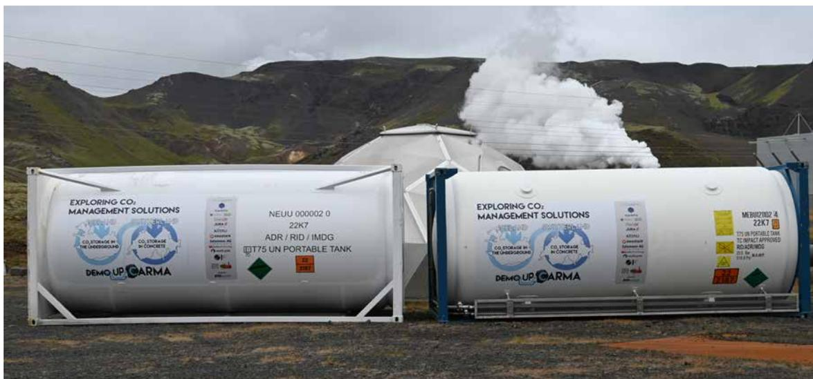
The liquefied CO<sub>2</sub> is transported from Switzerland to Iceland in special containers by truck, train and ship (source: DemoUpCARMA/ETH Zurich).
