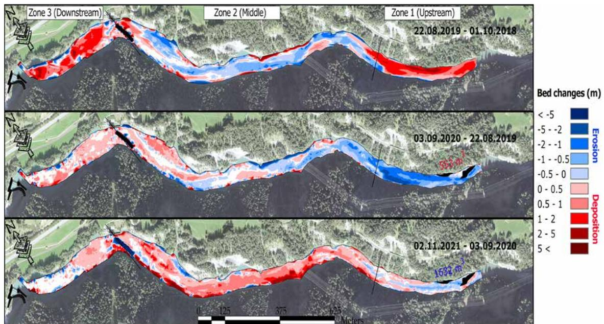
A result from the research project: bedload deposition (red) and bedload erosion (blue) in the Solis reservoir for three periods in the period from 2018 to 2021. The black dotted line in the lower area of the reservoir indicates the tunnel inlet (flow direction: from right to left; source: VAW ETH Zurich, edited).
