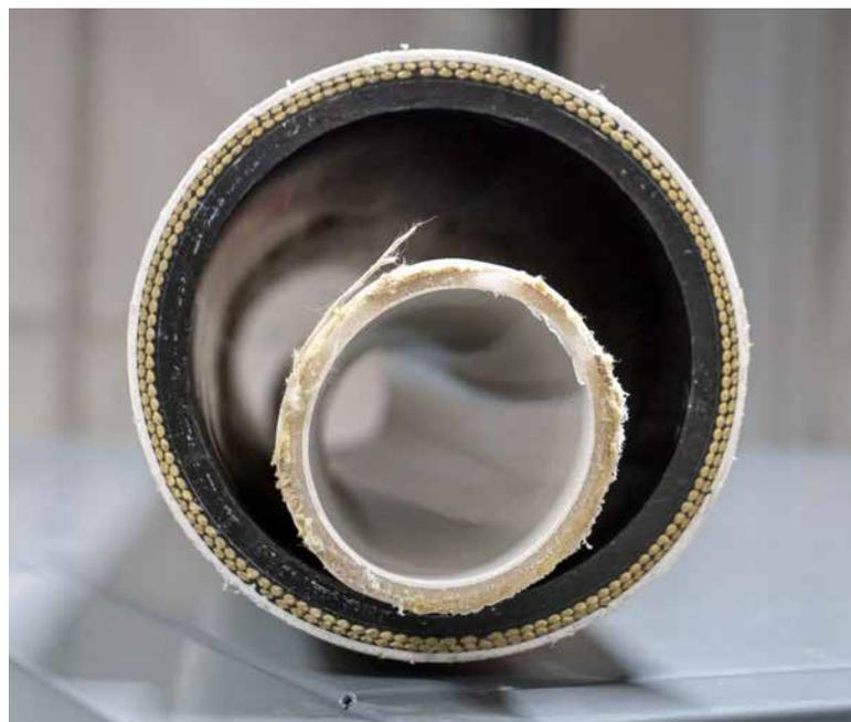
The inner pipe carrying the CO<sub>2</sub> is surrounded by another pipe for safety reasons. Both pipes can withstand a pressure of 90 bar (source: HES-SO Valais-Wallis).
