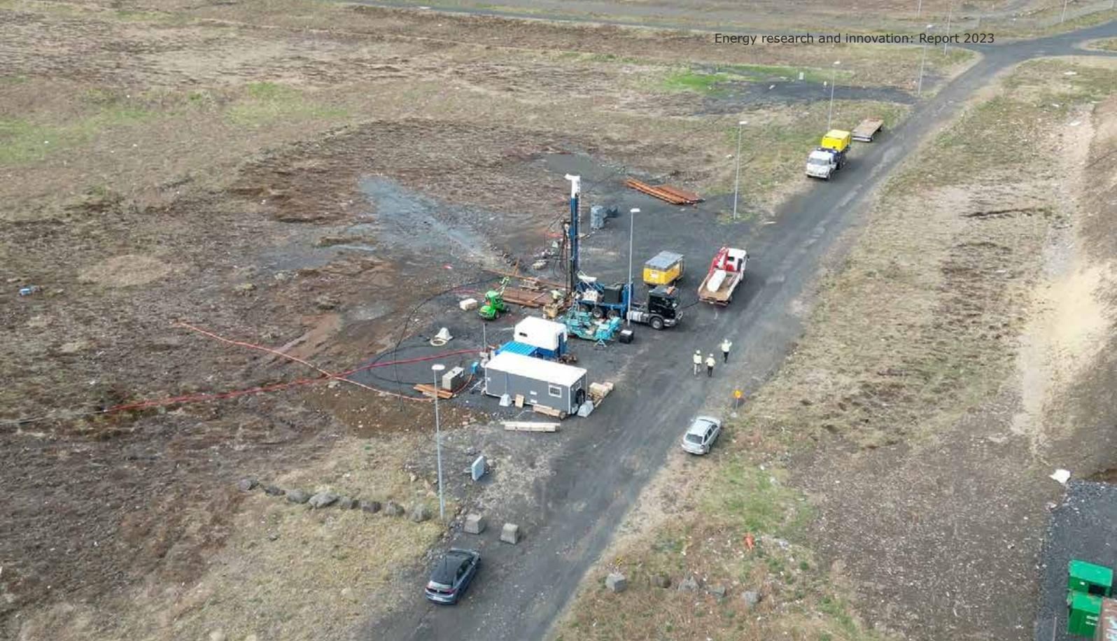
At two locations in Iceland, the CO<sub>2</sub> is mixed with fresh water and, for the first time, with seawater and injected into the basalt (source: DemoUpCARMA/ETH Zurich).
