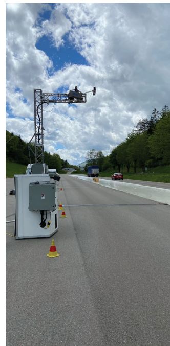
The EDAR measurement system during the project test phase in Switzerland. Illustration: Empa/In-NET Monitoring AG, 6460 Altdorf
