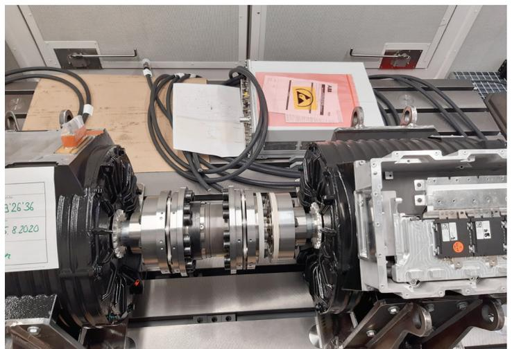
The Roadrunner project, in which bus manufacturer Hess and the ABB Group are developing a converter based on WBG semiconductors, was launched in 2019. The photo on the left shows a prototype of the converter. The picture on the right shows the test bench on which, among other things, journeys can be simulated. Photos: ABB Schweiz AG
