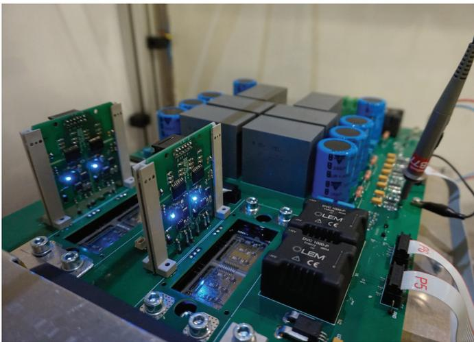
The team of Prof. Dr. Nicola Schulz has built and tested a DC-DC converter (22 kW; DC voltage 700 V to DC voltage 400 V) based on SiC at the University of Applied Sciences Northwestern Switzerland (Windisch site) in a project supported by the SFOE. Photo: FHNW
