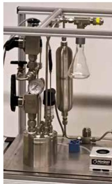
(Right) Laboratory prototype of an aluminium converter for hydrogen production in combination with a 12 W fuel cell (source: SPF).
