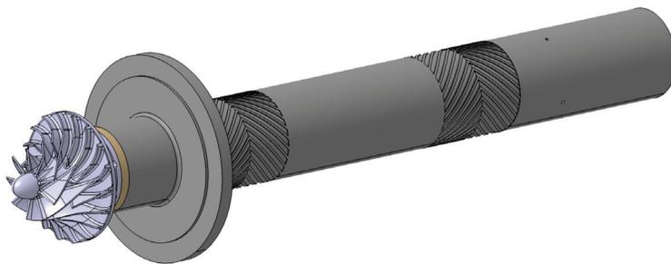
CAD representation of the rotor of a radial compressor: The bladed impeller is at the front, which radially deflects the heat pump's gaseous working fluid (flowing in from the left). The rotor is outfitted with V-shaped grooves, which create a gas film through the rotational movement, so that the rotor «floats» without touching the moving parts. Illustration: LAMD
