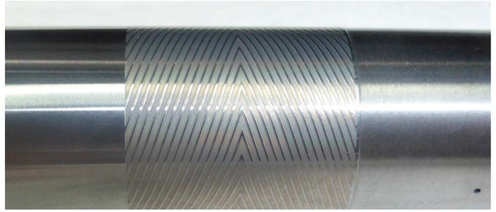
The V-shaped grooves are laser-etched into the steel rotor. The pattern of the grooves has been chosen so that the air gap between the rotor and bearing is as large as possible, due to operational advantages. Illustration: LAMD
