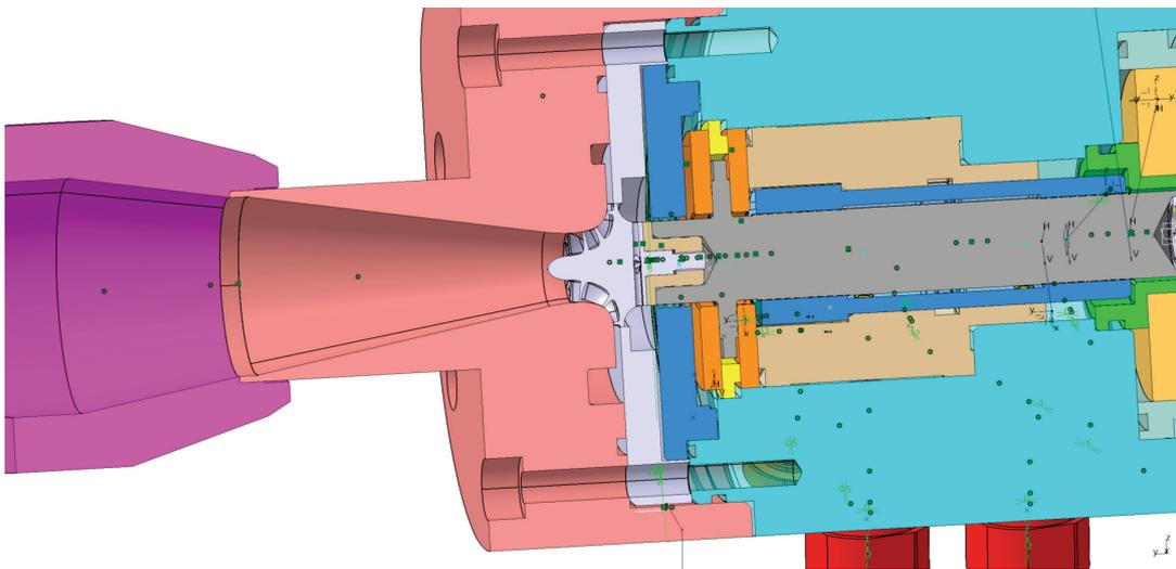
Cross-sectional view of a centrifugal compressor: The gaseous refrigerant reaches the compressor impeller via an inlet cone (light grey in the middle of the picture). The impeller transfers kinetic energy to the working fluid (energy of movement) and deflects it laterally. Graphic: LAMD
