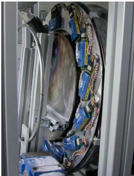
**Fig. 2:** Close view of the mini telemetry system consisting of eight modules mounted on a plate at the rear of the rotary reactor. The electronic components are cooled with air jets.
