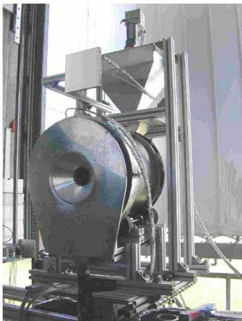
**Fig. 1:** The indirect-heated 10-kW solar lime prototype reactor mounted on the experiment table in the Small Solar Furnace at PSI. The experimental set-up comprises the rotary kiln, which is protected with a water-cooled shield, a white target for solar flux measurements, a reactants feeding and a product discharging system.
