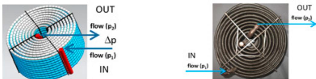
Figure 2: 3D CAD view and photo of the corrugated spiral tube Evaporator-Condenser (E-C) with the Copper (Cu) fluid headers in red. The heat transfer fluid flow indication stem from the pressure loss ( $\Delta p=p_1-p_2$ ) measurement.
